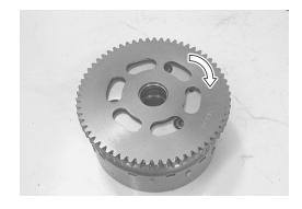
• Inspect the starter driven gear bushing for any damages.
