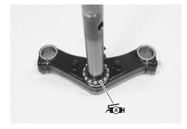
• Tighten the steering stem nut.
