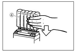
Make sure air bubbles (5) are coming up each electrolyte container, and leave in this position for about more than 20 minutes.
