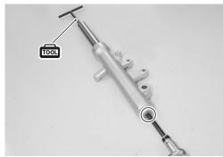
• Remove the inner tube ⑤ and oil lock piece ⑥ from the outer tube.
