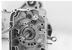
• With the crankshaft held immovable, loosen the crankshaft right bearing nut using the special tool.
