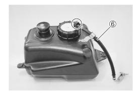
• Loosen the fuel pump retainer using the special tool.
