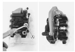
• Blow the hole (B) to push out the upper and lower pistons.
