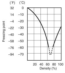
Fig. 1 Engine coolant density-freezing point curve
