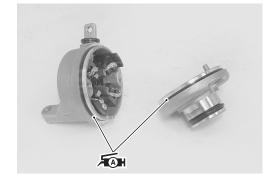
• Fit the washer ① to the housing end with the tabs aligned with the housing end cutaways, position the shim ② and assemble the starter motor.
