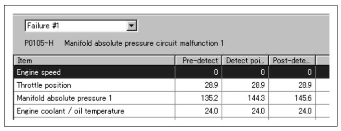
• Click "Show data when trouble" ① to display the data. By clicking the drop down button ②, either "Failure #1" or "Failure #2" can be selected.
