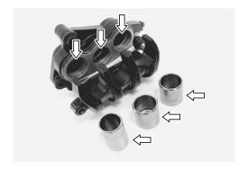
Inspect the caliper bracket 1 for any damage. Inspect the rubber boots 2 for any damage. If any abnormal condition is noted, replace it with a new one.
