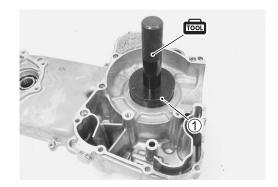
Install new oil seal ② using the special tool.
