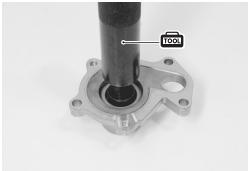
Apply a small quantity of grease to the oil seal lip.
