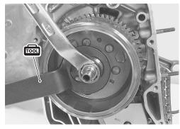
• Remove the generator rotor ③ and starter driven gear ④ using the special tool.
