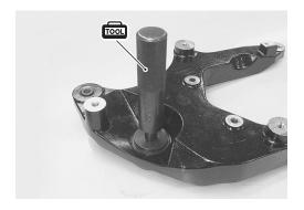
• Install new dust seal using the special tool.
