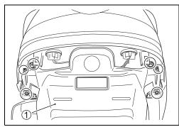
• Turn the socket counterclockwise and remove it.
