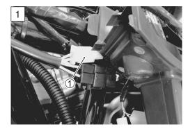
4) Disconnect the CKP sensor coupler and measure the resistance.
