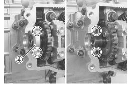
• Remove the camshaft sprocket bolts.
