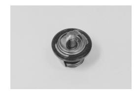
• Immerse the thermostat in water contained in a pan as shown and measure the valve start-to-open temperature when water is heated gradually.
