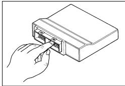
When disconnecting and connecting the ECM, make sure to turn OFF the ignition switch ①, or electronic parts may get damaged.
