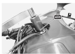
• Tighten the handlebar set bolt ③ and handlebar clamp nut ④ to the specified torque.
