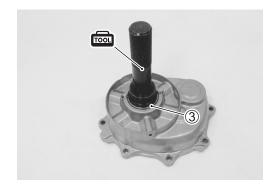
• Install the bearing retainer ④ toward the upper side ④ of the engine
