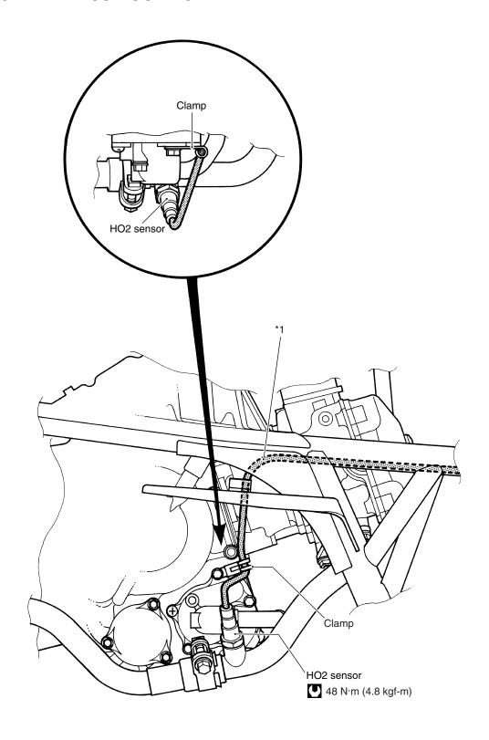
Pass the HO2 sensor lead wire between the \*1 frame and engine. Do not protrude the HO2 sensor lead wire from the frame.
