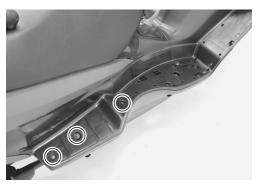
• Remove the rear combination light ②, upper frame cover ③ and rear footboards ④ (LH and RH) from the frame covers ⑤ (LH and RH).
