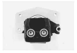
• Tighten the brake caliper mounting bolts ①.
