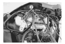
• Remove front box ④ along with the speedometer and lower meter panel.
