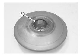
• Remove the needle bearing using the special tool.
