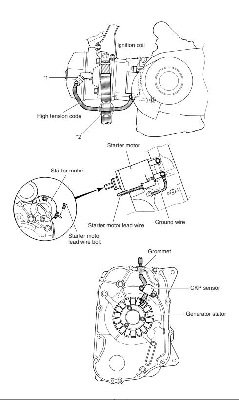
\*1 Bring the tip of spark plug cap to downward.
