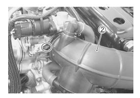
• Disconnect the engine ground wire ③ and starter motor lead wire 4.
