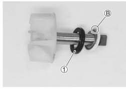
• Install the water pump shaft and the E-ring 2.
