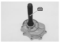
• Install the bearing ③ using the special tool.
