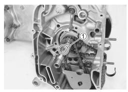
• Install the generator rotor ② together with the starter driven gear ③.
