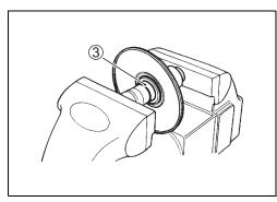
• Apply grease to both bearings.
