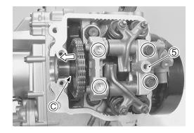
• Remove the camshaft ⑥ and camshaft sprocket.
