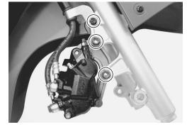
• Remove the speed meter cable guide ①.
