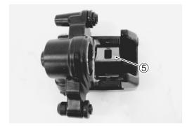
Using an air blow gun, pressurize the caliper fluid chamber to push out the piston.
