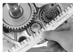
• If the measured clearance is not within the specification, measure the thickness of the shim ① with the micrometer and select the specified shim from the table below.
