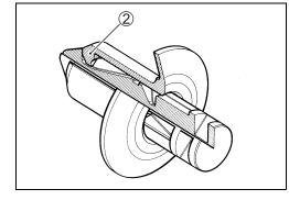
• Push in the head of center piece until it becomes flush with the fastener outside face.
