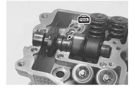
Tighten the camshaft journal holder bolts evenly and diagonally to the specified torque.
