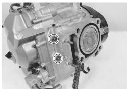
• Remove the cylinder gasket 2 and dowel pins.
