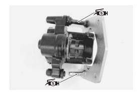
Install the brake pads and brake pad bolts.
