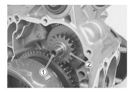
• With the generator rotor held immovable with the special tool, remove the generator rotor nut.
