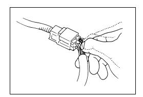
When taking measurements at electrical connectors using a tester probe, be sure to insert the probe from the wire harness side (backside) of the connector/coupler.
