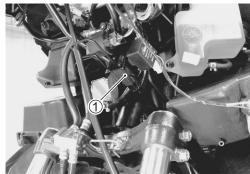
Check that no continuity exists between the terminals 2 and 3. If continuity is found, replace the relay.
