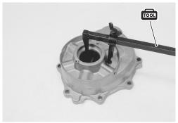
• Remove the bearing ④ using the special tool.
