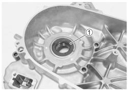
• Remove the bearing ② using the special tool.
