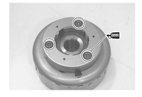
$\bullet$  Remove the generator stator 1 and CKP sensor 2.
