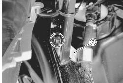
• Remove the fuel tank bolt 3.
