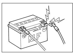
Before measuring voltage at each terminal, check to make sure that battery voltage is 11 V or higher. Terminal voltage check with a low voltage battery will lead to erroneous diagnosis.
