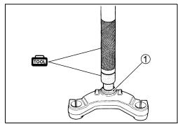
Apply grease to the upper bearing and upper inner race prior to installing the steering stem.
