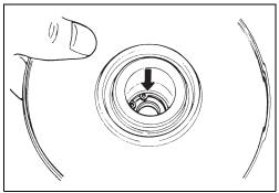
• Install needle bearing ③ using an appropriate specer.
