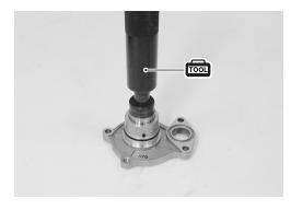
• Install the oil seal with the special tool.
