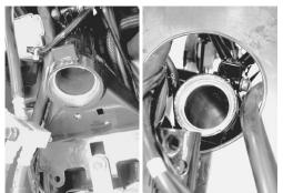
To remove the lower inner race, use a chisel like, plain head steel rod.
