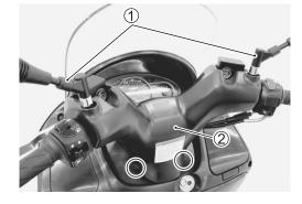
• Remove the front handlebar cover 3.
