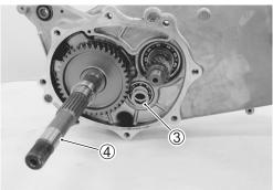
• Remove the driveshaft ⑤ by tapping it with a plastic mallet.
