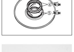
• Install the movable driven face (6) to the fixed driven face (2).
