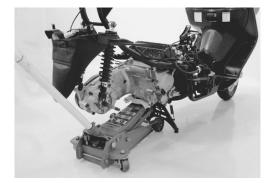
• Remove the rear shock absorber mounting bolt (LH).
