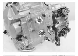
• Remove the cylinder head bolts.
