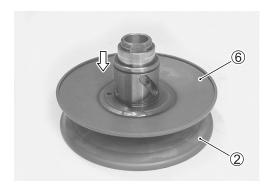
• Install the movable driven pins 7 and rollers to the pin holes with grease coated.
