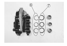
Inspect the caliper cylinder wall and piston surface for scratch, corrosion or other damages.
