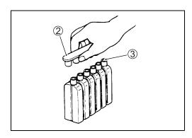
• Insert the nozzles of the electrolyte container ④ into the battery's electrolyte filler holes, holding the container firmly so that it does not fall. Take precaution not to allow any of the fluid to spill.
