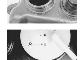
• Tighten the fuel pump retainer using the special tool.
