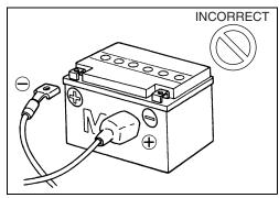
Removing any battery terminal of a running engine is strictly prohibited.
