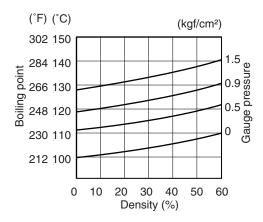
Fig. 2 Engine coolant density-boiling point curve
