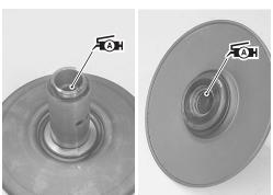
• Install the oil seals 4 and O-rings 5 to the movable driven face.
