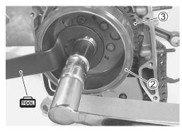
• Install the starter idle gear 1 and starter idle gear shaft 2.
