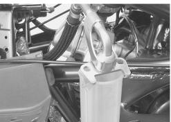
• Disconnect the fuel pump lead wire coupler 2.
