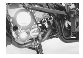
• Install the insulator and throttle body assembly.
