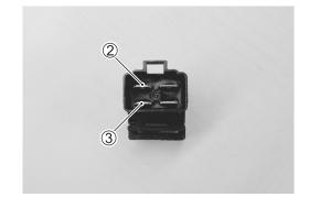
Check there is continuity between the terminals ② and ③ when 12 V battery voltage is applied; positive to the terminal ④ and negative to the terminal ⑤. If no continuity is noted, the relay must be replaced.
