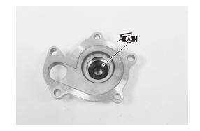
• Install the new mechanical seal using a suitable size socket wrench.
