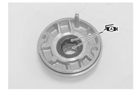
Apply a little SUZUKI MOLY PASTE to the armature shaft end.
